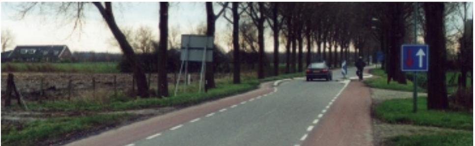
Yes, traffic calming not in town but in the middle of the country! Past the cyclist and motorist is a major, for this road, junction. Though the single motor vehicle lane gives room to the cyclists on straight stretches of road it doesn't limit speed – thus the use of a chicane to slow traffic down. Note that the cyclists are provided with bypasses on either side of the chicane so they are not squeezed by cars trying to taking the chicane too fast.
